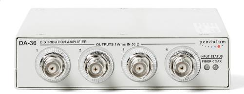
The Pendulum DA-36 frequency Distribution Amplifi er offers an economical solution to the problem of low-jitter transfer of frequency reference signals over longer distance. Whether the need is to distribute between remote buildings, fl oors or rooms, or whether the need is a big point-to-multipoint system with thousand of receivers, or just one single point-to-point distribution, DA-36 will do the job.
