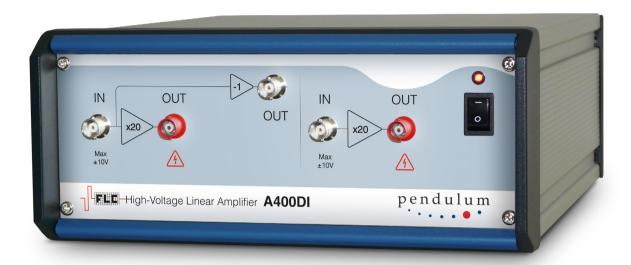
The Pendulum Instruments Dual Channel High Voltage Linear Amplifier A400DI contains two independent A400 amplifiers that share common ground reference and power supply. It features also a low voltage phase inverter that inverts the signal applied to the input of channel 1. The resulting signal can then be connected to the input of channel 2 by means of a short BNC cable (supplied).
