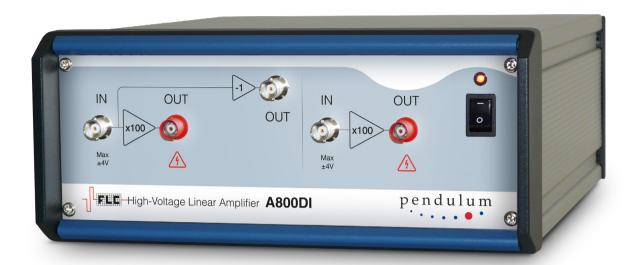
The Pendulum Instruments Dual Channel High Voltage Linear Amplifier A800DI contains two independent A800 amplifiers that share common ground reference and power supply. It features also a low voltage phase inverter that inverts the signal applied to the input of channel 1. The resulting signal can then be connected to the input of channel 2 by means of a short BNC cable (supplied).
